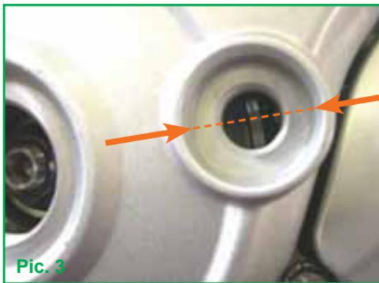
Turn the crankshaft counterclockwise using the generator rotor nut until you find the right position.
