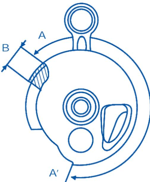
A-A' = 190 mm (measured on the disc external diameter)
